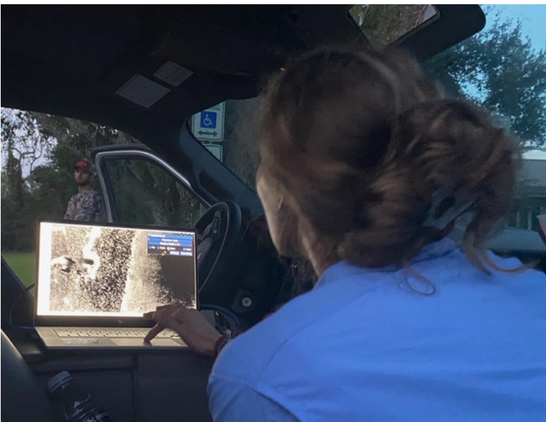
A live Burmese python viewed on a computer screen using a 850nm near-infrared camera.
